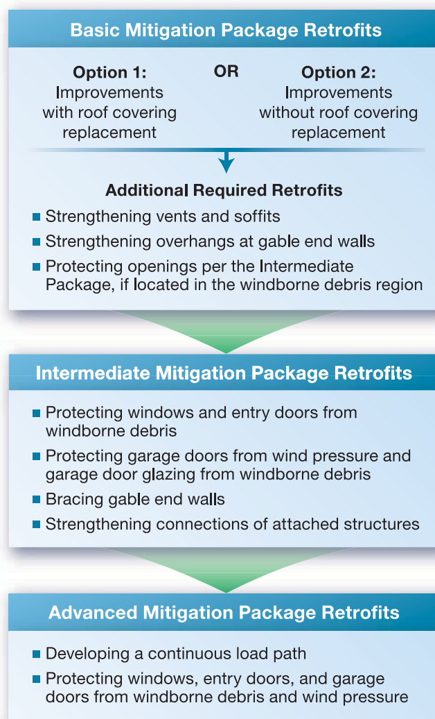
Figure 15-15. Wind Retrofit Mitigation Packages
