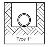
Type 1 pipe laying requires excavation of earth below pipe bell so the pipe bears uniformly upon undisturbed native earth. Soil is backfilled and tamped by hand around the pipe (and completely under the pipe haunches) in uniform layers not exceeding six inches in depth.
