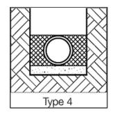
At a minimum, Type 4 laying condition shall be utilized with a minimum of 6-inches of bedding to overcome unstable conditions. For severe unstable soil conditions, undercut excavation and an engineer designed foundation plan shall be provided prior to pipeline installation.
