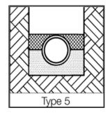
Type 5 laying condition shall be utilized for gravity sewer and pipelines greater than 8 -inch diameter with >14 feet to 20 feet of cover and where rock or other hard, angular materials are encountered. The City Inspector may require Type 5 in other cases to overcome unstable conditions.
